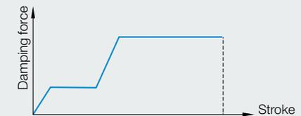
Controlled multi-stage closing: initial low force prevents re-bounce, followed by higher force for efficient deceleration
